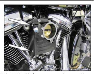
6. Install the K&N® servo cover and secure with the provided hardware to the original servo cover mounting bolt locations.
