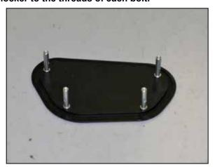
11. Install the four provided spacer bolts and washers into the filter top plate as shown. NOTE: Apply one drop of the provided thread locker to the threads of each bolt.
