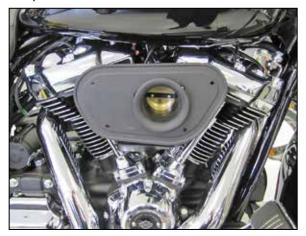
10. Using the three provided throttle body bolts, secure the filter back plate to the base plate as
