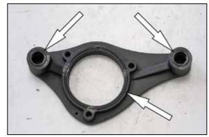
7. Install two of the breather O-rings and the throttle body O-ring into the base plate as shown. NOTE: Use a few small dabs of grease to secure the O-rings in place while installing the
